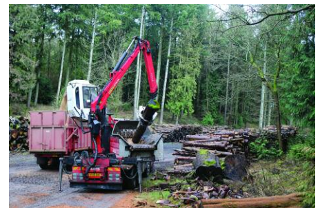
The Wood Terminator 10XL munches its way effortlessly through 75cm diameter trunks of diseased ash.
